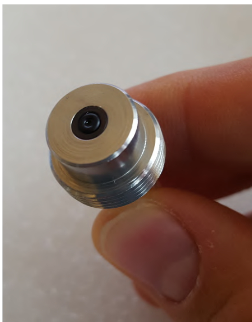
(A) For 25 - 1000 \mu\text{L} syringes, ensure that the black O-ring is correctly inserted in the groove as shown here
