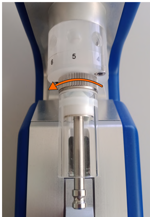
(B) Syringe removal for 2.5 - 5 mL syringes
