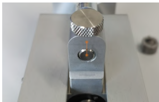
FIGURE 4.11 – Alignment to be obtained when screwing the plunger lock screw
