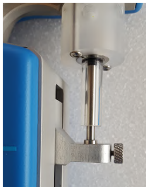
FIGURE 4.13 – Incorrect plunger lock screw fixation
