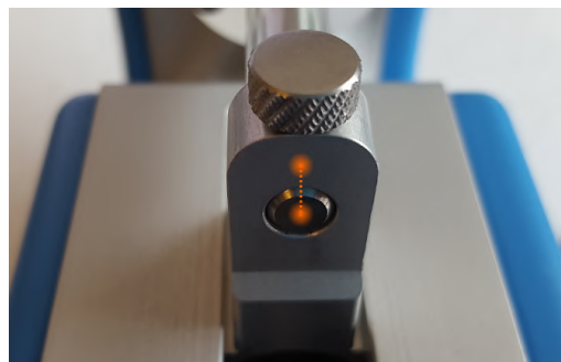
FIGURE 4.12 – Alignment to be obtained when screwing the plunger lock screw
