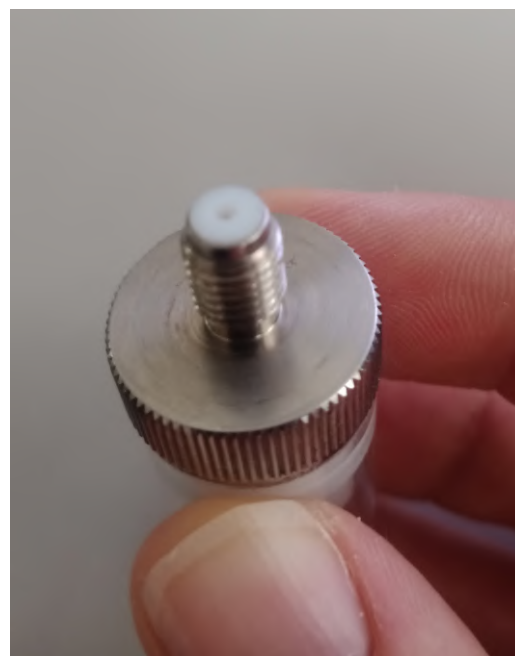
(B) For 2.5 - 5 mL syringes, ensure that the PTFE surface is clean and not scratched
