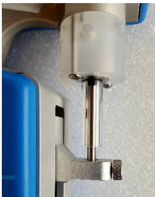
FIGURE 4.13 – Correct plunger lock screw fixation
