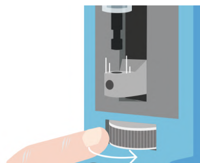
FIGURE 4.5 – Move the slider down, using the driving wheel
