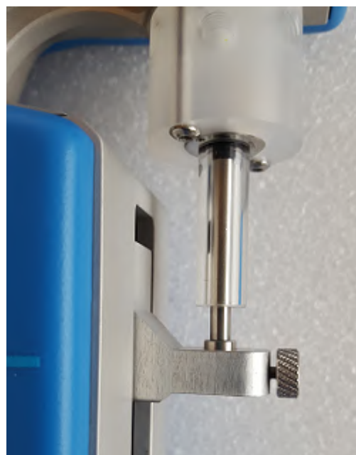
FIGURE 4.14 – Incorrect plunger lock screw fixation
