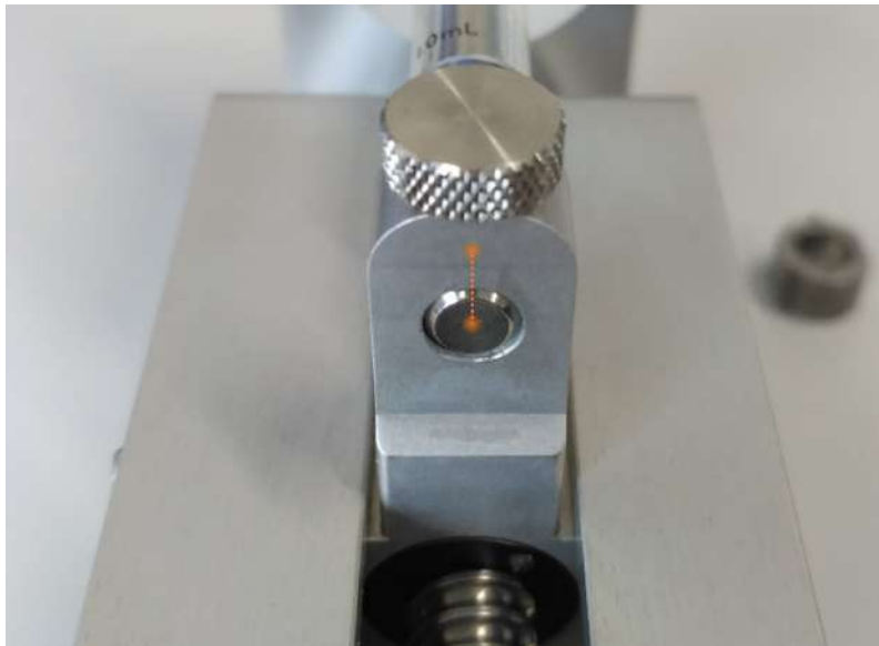
FIGURE 4.7 – Alignment to be obtained when screwing the plunger lock screw
