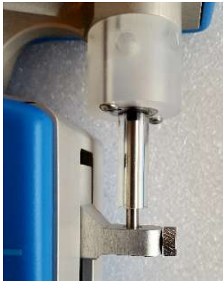
FIGURE 4.8 – Correct plunger lock screw fixation
