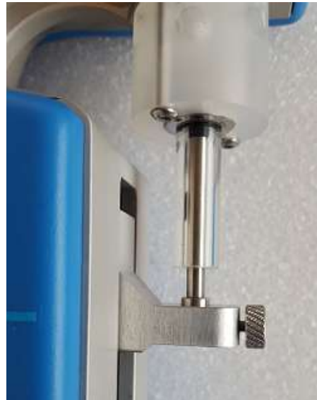
FIGURE 4.9 – Incorrect plunger lock screw fixation
