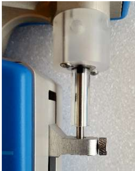
FIGURE 4.8 – Correct plunger lock screw fixation
