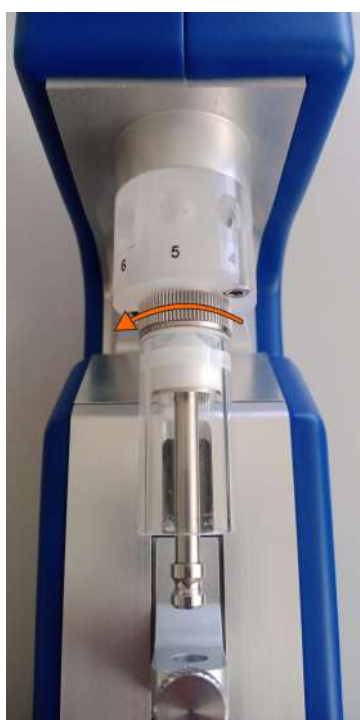
FIGURE 4.5 – Unscrew the syringe using fingers friction against the knurl
