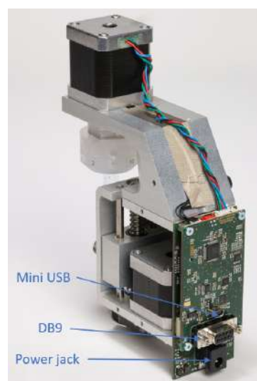
FIGURE 1.4 – SPM syringe pump terminology 2/2
