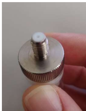
FIGURE 4.6 – Syringe seal to be handled with care. Before screwing the syringe, ensure that the PTFE surface is clean and not scratched
