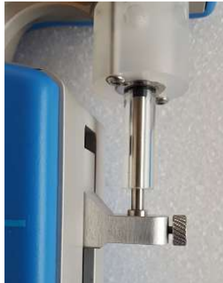
FIGURE 4.9 – Incorrect plunger lock screw fixation
