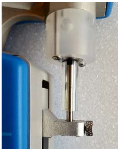
FIGURE 4.6 – Correct plunger lock screw fixation
