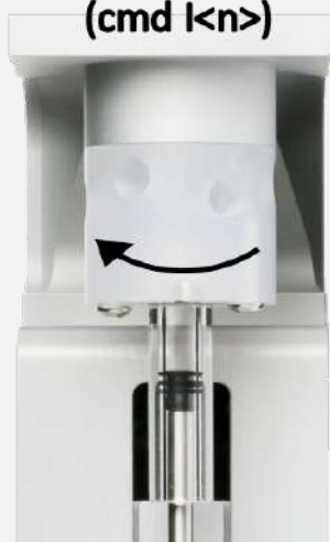
FIGURE 3.7 – Direction of rotation definition for the plug - clockwise rotation corresponds to a 60° rotation when incrementing the port number by 1, counterclockwise rotation corresponds to a 60° rotation when decrementing the port number by 1
