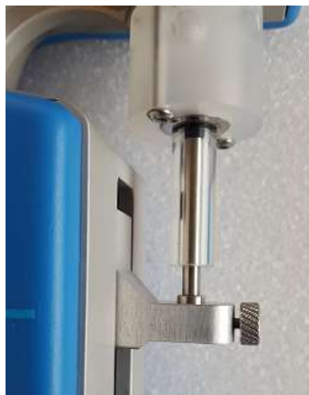
FIGURE 4.7 – Incorrect plunger lock screw fixation
