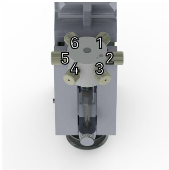
FIGURE 3.2 – Cut section revealing port numbering - VD1-6
