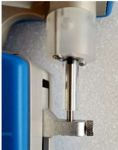
FIGURE 4.6 – Correct plunger lock screw fixation
