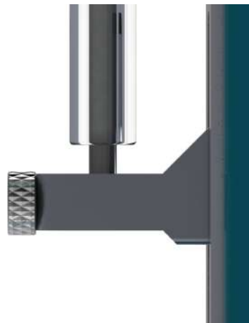
FIGURE 1.3 – Detail of plunger fixation when correctly tightened
