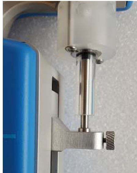
FIGURE 4.7 – Incorrect plunger lock screw fixation
