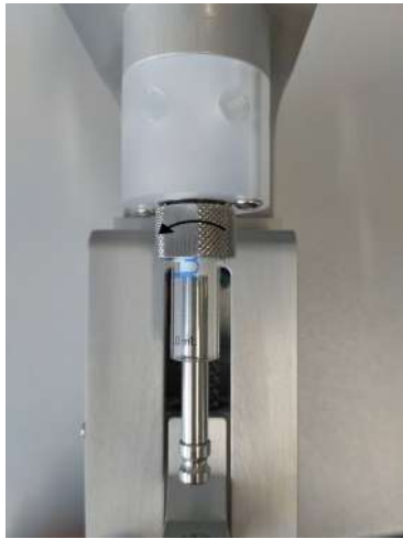
FIGURE 4.3 – Insertion of the syringe removal tool around the glass barrel. Unscrew the syringe by turning in the highlighted direction.
