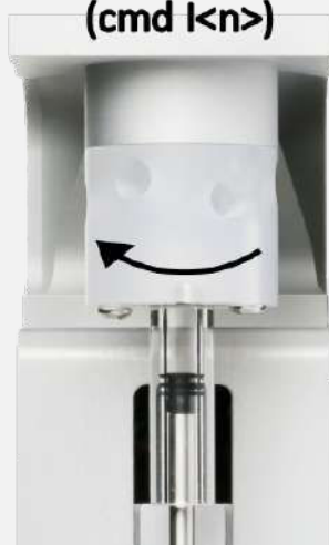
FIGURE 3.7 – Direction of rotation definition for the plug - clockwise rotation corresponds to a 60^\circ rotation when incrementing the port number by 1, counterclockwise rotation corresponds to a 60^\circ rotation when decrementing the port number by 1
