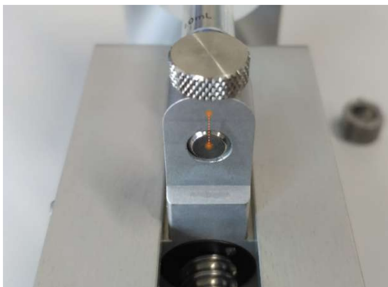
FIGURE 4.5 – Alignment to be obtained when screwing the plunger lock screw
