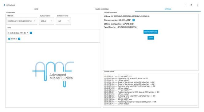
The settings tab allows you to input which specific pump configuration you are using:
