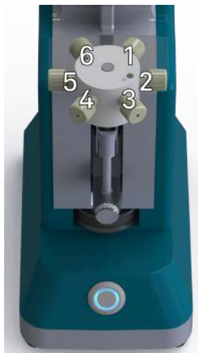
FIGURE 3.2 – Cut section revealing port numbering - VD1-6
