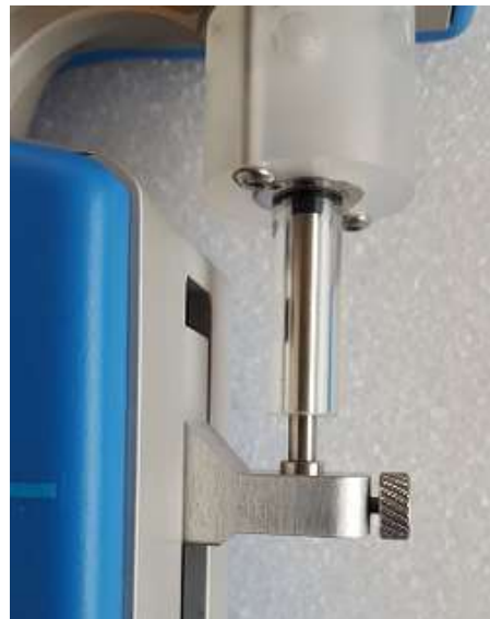
FIGURE 4.10 – Incorrect plunger lock screw fixation
