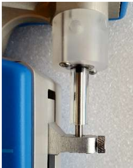
FIGURE 4.9 – Correct plunger lock screw fixation
