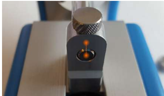
FIGURE 4.8 – Alignment to be obtained when screwing the plunger lock screw
