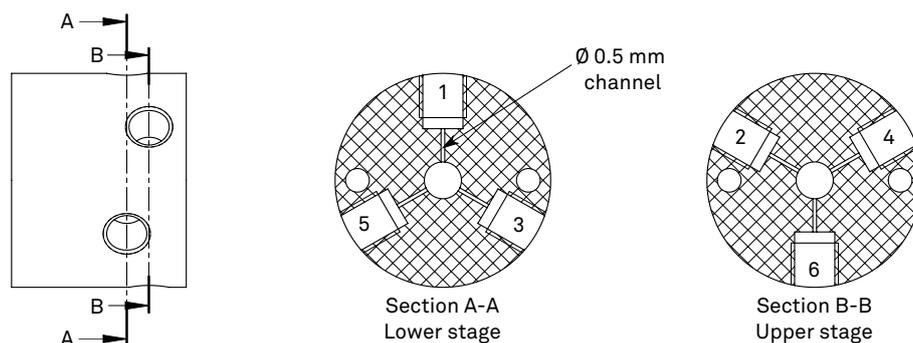
FIGURE 3.6 – Section view of the PCTFE valve seat with port numbering
