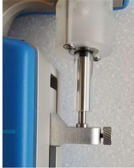
FIGURE 4.8 – Incorrect plunger lock screw fixation
