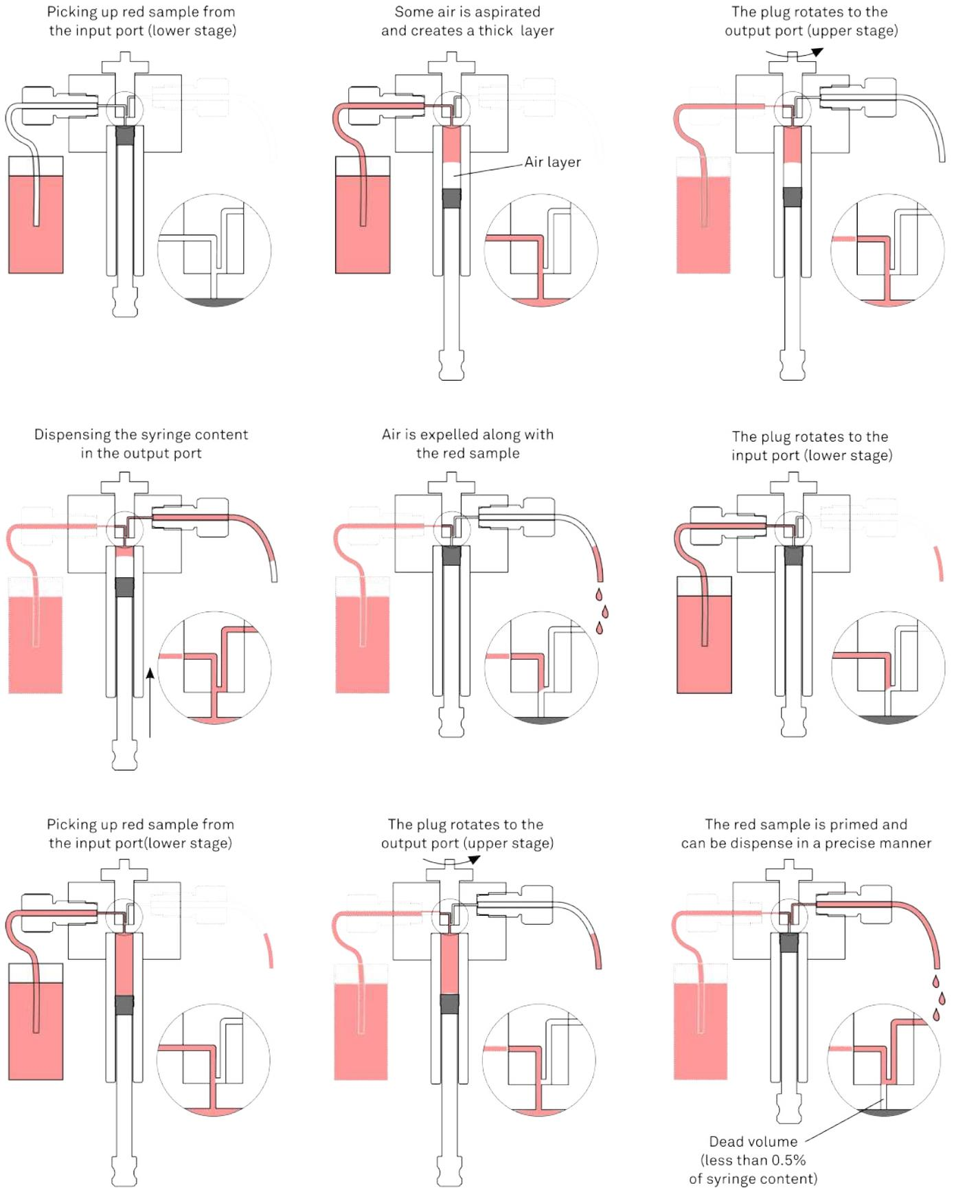
FIGURE 3.9 – Automated priming process with LSPone
