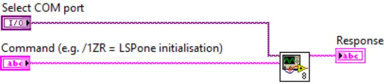
FIGURE 8.2 – Labview sub-VI,bloc diagram - 1 pump
