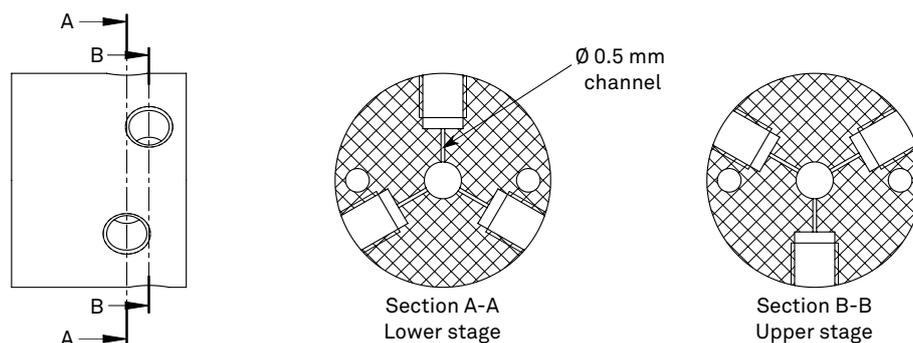
FIGURE 3.4 – Section view of the PCTFE valve seat revealing the microchannels - VD2-6
