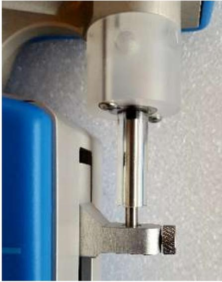
FIGURE 4.7 – Correct plunger lock screw fixation
