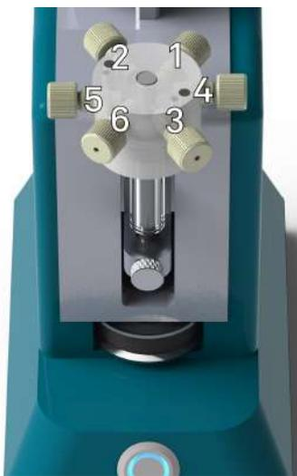
FIGURE 3.5 – Cut section revealing port numbering - VD2-6
