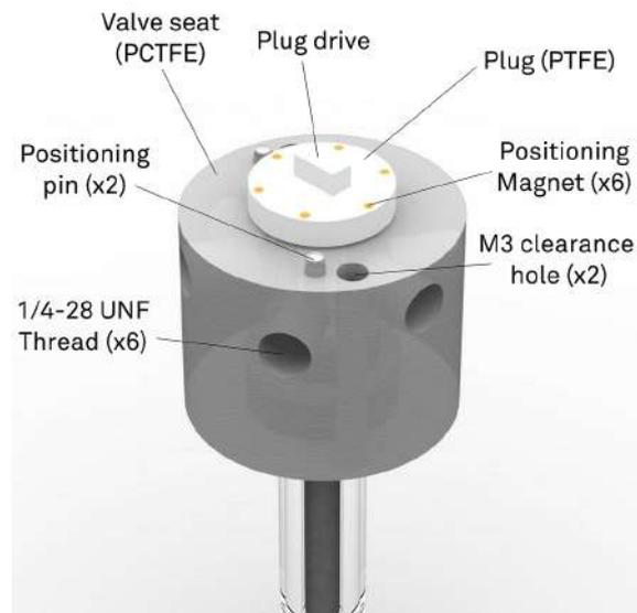
FIGURE 1.5 – Nomenclature for the valve module
