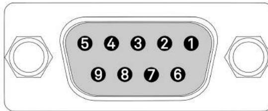
FIGURE 2.4 – DB9 pin-out on device side (LSPone)
