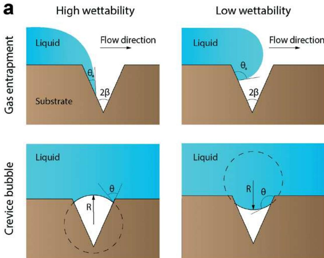
FIGURE 4.1 – Image that describe the formation of bubble due to a crevice during the wetting of the microfluidic network (source : Pereiro, Iago, et al. "Nip the bubble in the bud: a guide to avoid gas nucleation in microfluidics." Lab on a Chip 19.14 (2019): 2296-2314)
