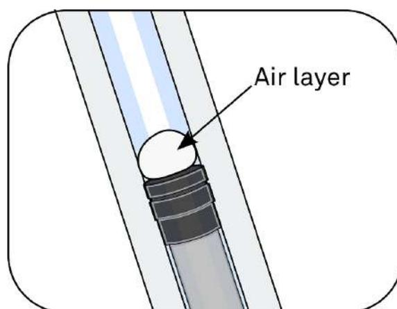
FIGURE 3.8 – Air layer appearing with conventional syringe pumps
