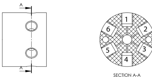
FIGURE 3.3 – Section view of the PCTFE valve seat with port numbering - VD1-6
