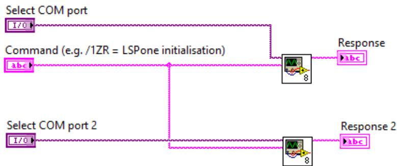
FIGURE 8.4 – Labview sub-VI, bloc diagram - 2 pumps
