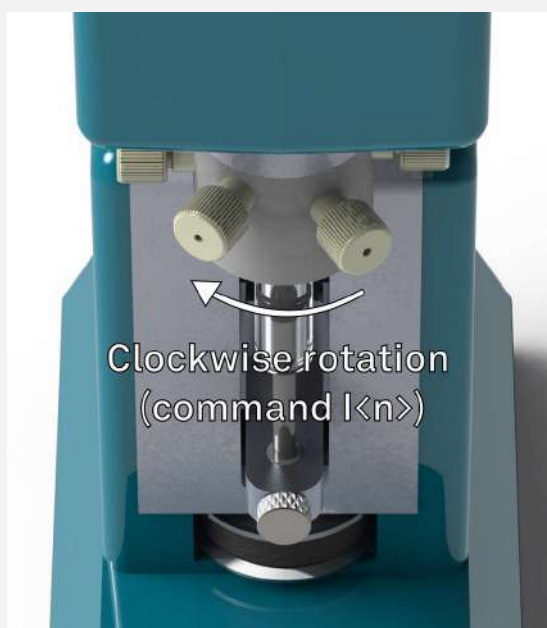
FIGURE 3.7 – Direction of rotation definition for the plug - clockwise rotation corresponds to a 60° rotation when incrementing the port number by 1, counterclockwise rotation corresponds to a 60° rotation when decrementing the port number by 1
