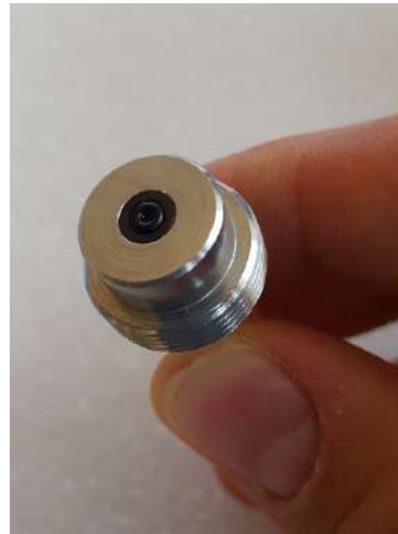
FIGURE 4.5 – Syringe seal to be handled with care. Before screwing the syringe, ensure that the black O-ring is correctly inserted in the groove as shown here
