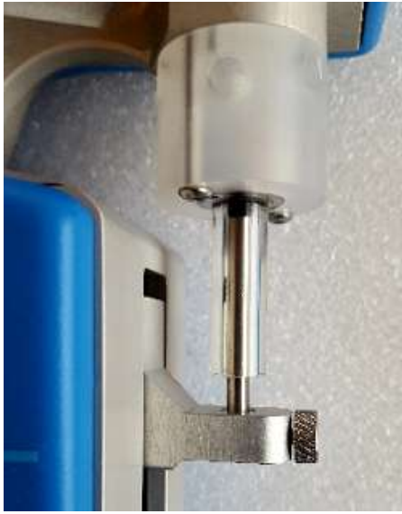
FIGURE 4.7 – Correct plunger lock screw fixation
