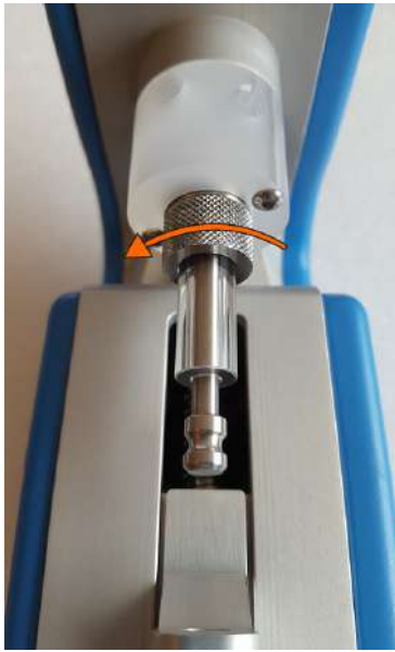
FIGURE 4.4 – Insertion of the syringe removal tool around the glass barrel. Unscrew the syringe by turning in the highlighted direction.
