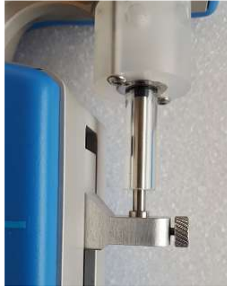
FIGURE 4.8 – Incorrect plunger lock screw fixation
